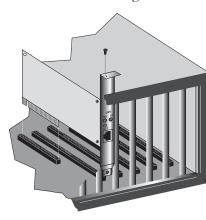
1. To install the EZ Card 10/100, power off your PC and remove the chassis cover. Next, select an unused PCI expansion bus slot and remove its protective bracket. Carefully insert the card and
