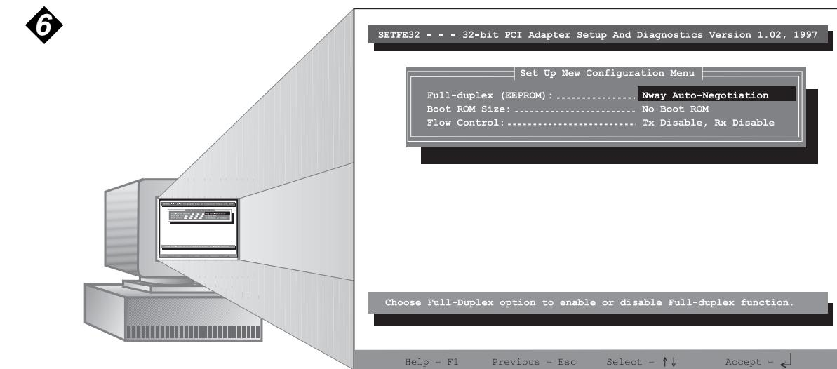
The host computer's BIOS automatically allocates the necessary resources to the EZ Card 10/100. Although the Setup Program will not allow you to change those resources, you can change the settings displayed on the "Setup New Configuration" screen (see above). Note: The Interrupt and I/O Base are controlled by the host computer's BIOS, not the Setup Program.
